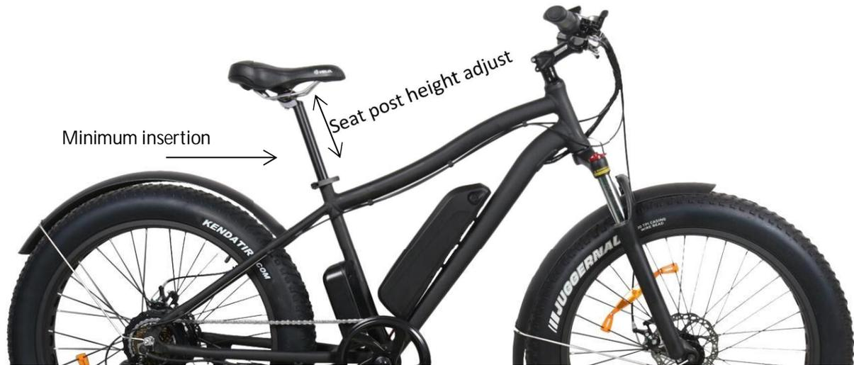
To adjust seat height, use quick release lever to set free the seat post and pull upwards or push downwards to reach desired height.
